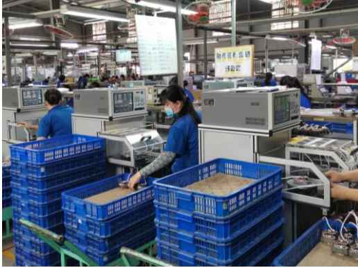
Stator winding test
