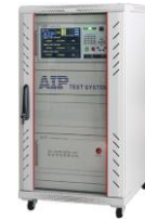
Stator wrong winding test
