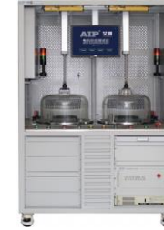
Stator vacuum test
