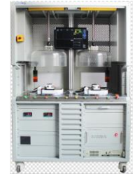
Coil point damage detect
